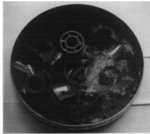
Fig. 5. Naturally-aged cellulose nitrate base cinematograph film in a severe state of deterioration; exhibiting loss and shrinkage of emulsion, crumbling of base and deposition of large volumes of a brown
